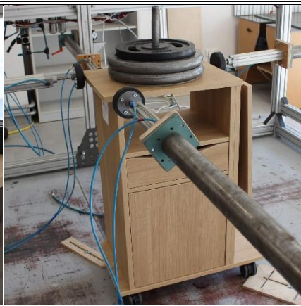
Figure 6: Horizontal durability test: - Load on the table top, 50 kg; - force 300 N; - cycles 20000.
