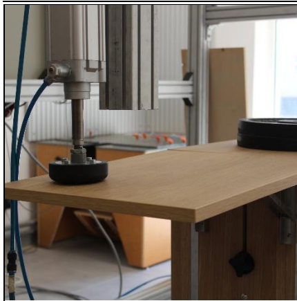
Figure 5: Vertical static load on ancillary surface: - force 200 N; - cycles 10.
