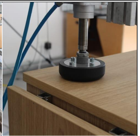
Figure 7: Vertical durability test: - force 300 N; - cycles 20000
